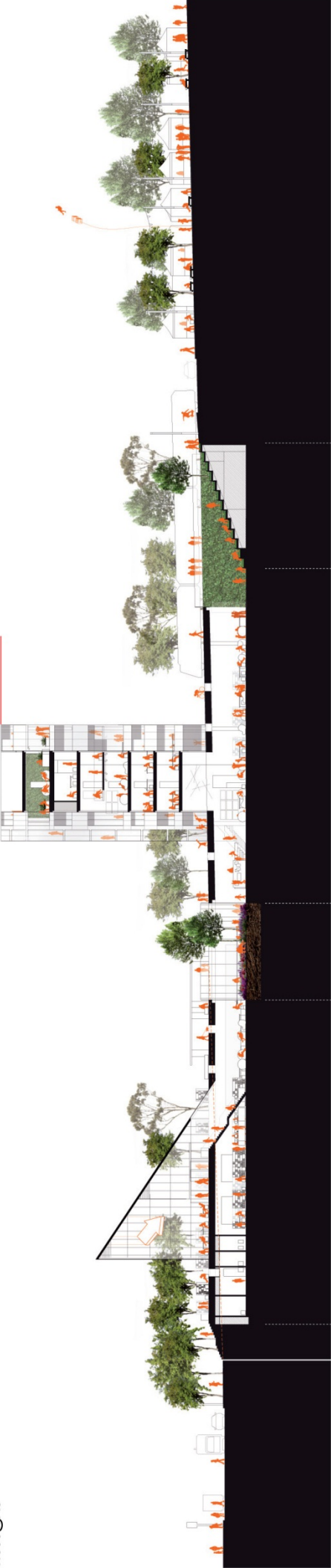
Library and Plaza design: Section illustrating maximum building height envelope of RL46.0
